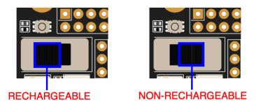
Figure 9: Battery selector switch
