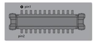
Figure 12: WisBlock 24-pin module connector
