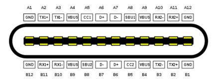
Figure 4: USB Type-C receptacle pinout
