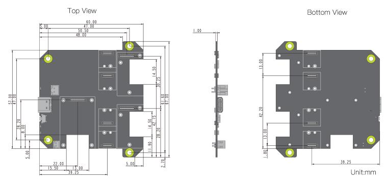
Figure 14: RAK19001 board dimensions
