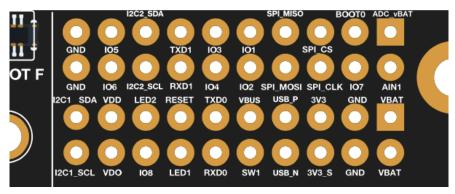
Figure 5: J10 and J15 pin header label in bottom side
