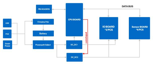
Figure 2: RAK19001 WisBlock Base block diagram
