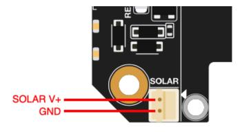
Figure 10: Solar panel connector V+ and GND
