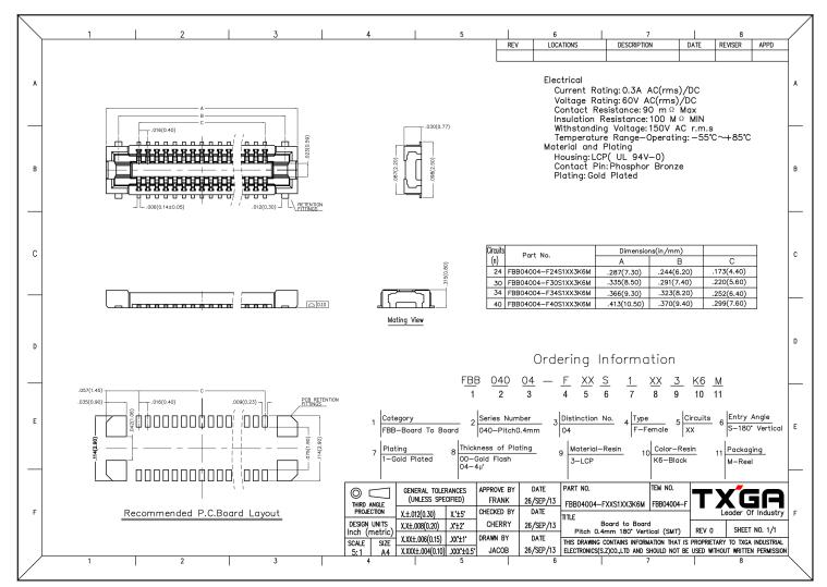
Figure 16: WisConnector PCB footprint and recommendations
