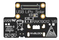
Figure 1: RAK19012 WisBlock Power Module top (left) and bottom (right) view
