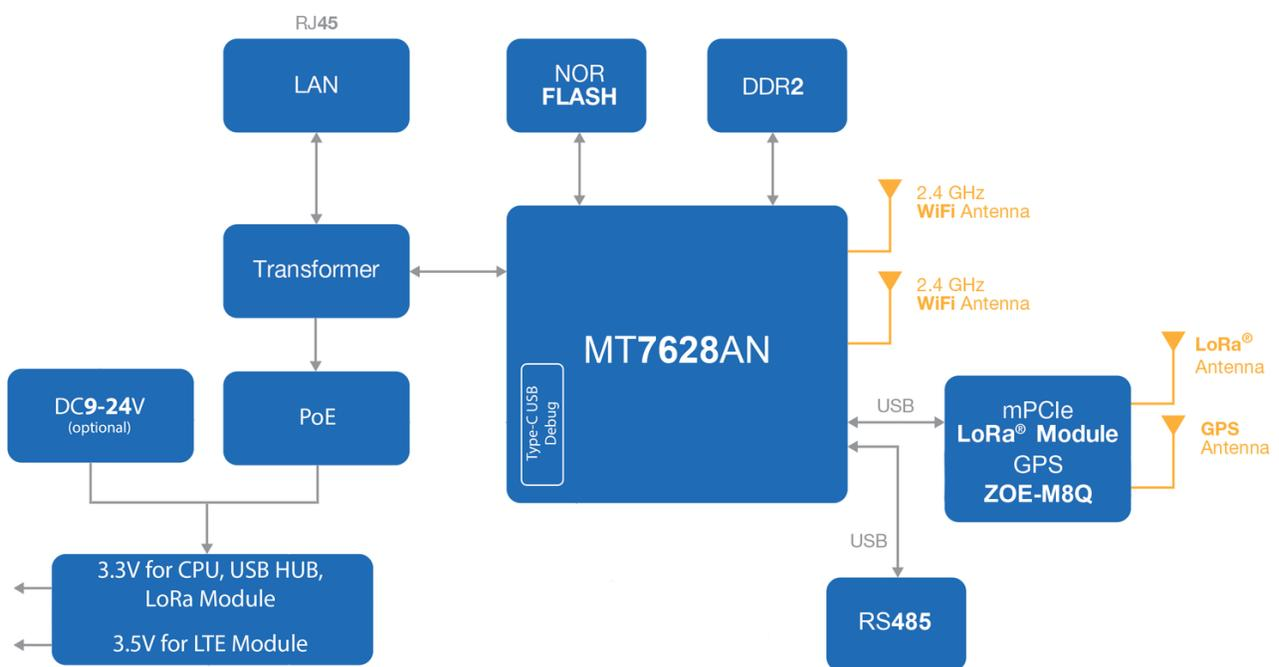
Figure 1: RAK7240V2 Block Diagram
