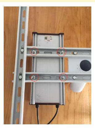
Figure 22: Mounting the Battery to the Bracket
