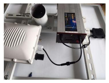
Figure 25: Lithium Battery Output Cord to RAK7249 - Marco Outdoor Gateway Connection
